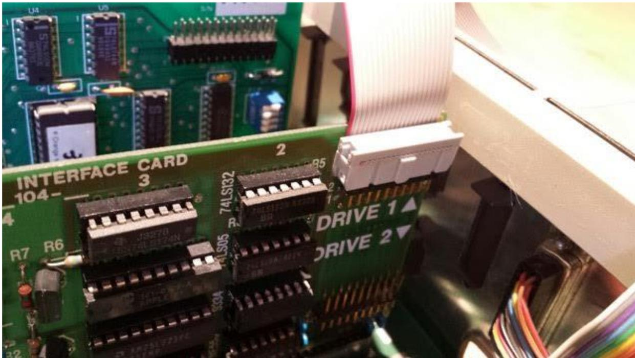
Pay careful attention to the cable orientation when connecting to a Disk II Controller Card in an Apple II computer. The Disk II connector lacks a polarity key, so it's easy to connect the cable backwards accidentally. This can result in damage to the Emu board or your computer. In the correct orientation, the red stripe on the cable will go to the pins marked “1” and “2” on the Disk II card, as shown in the photo. The cable will be sandwiched between the connector and the board.
