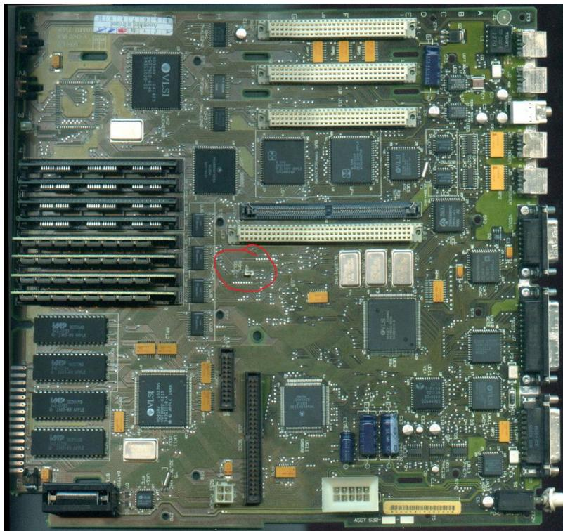
Figure 6 - Mac IIcx W1 Jumper Location
