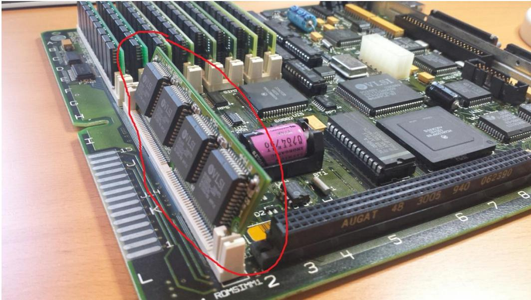
Figure 2 - Release Clips and Tilt SIMM Backwards
