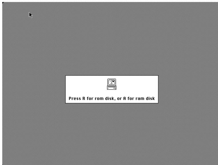
To boot from the ROM disk as a read-only disk, press the R key on the keyboard. Or to convert the ROM disk into a writable RAM disk, press the A key. Or to bypass the ROM disk, do nothing and wait five seconds. If no keys are pressed, the Macintosh will boot normally from an attached SCSI or HD20 disk, or will wait for a floppy disk to be inserted.
