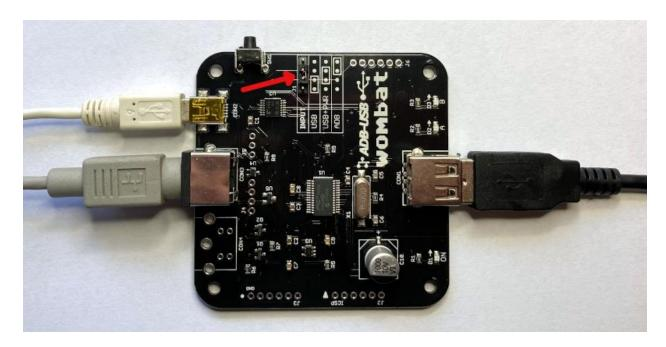
When in this mode, power for the Wombat will be supplied from the auxiliary power source, enabling the Wombat to keep running even when the computer is off. This enables the software-mapped keys PRINT SCREEN and F13 on a USB keyboard to be used as a power button to turn on a Macintosh computer, assuming the computer has a power supply that supports keyboard power switching.
