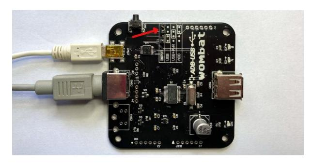
In this mode, power for the Wombat will be supplied from the USB host computer. The ADB peripherals will appear as standard HID input devices to modern Windows, OSX, and Linux computers. No special drivers or other software are needed. The Wombat supports one ADB keyboard and one ADB mouse.
