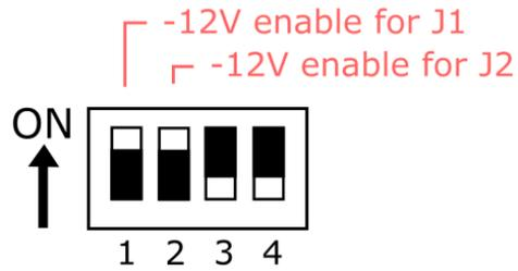
For 5.25 inch drives, and 3.5 inch drives in an external enclosure rather than naked, set the -12V DIP switch to the ON position.
